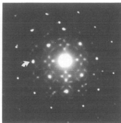
Fig. 1. Typical ED pattern of an \alpha phasoid crystallite found in a sample with nominal composition Ba_{0.8}Nb_4O_6 synthesized at 1200 °C. The ED pattern indicates a C-centred subcell with a \approx 4.2 Å. One subcell spot (200)_{\text{sub}} is arrowed. Around the subcell reflections, diffuse satellite spots are seen in two different directions depending on (h + k)_{\text{sub}} being even or odd.
